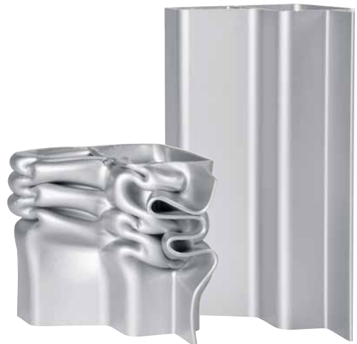
Multi-chamber profile offering good crash resistance
