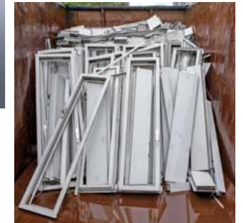
Well-functioning aluminium recycling loop: used profiles are collected (lower image) and the resultant aluminium scrap is turned into new window profiles. (left: Schüco AWS 90.SI+ Green)
