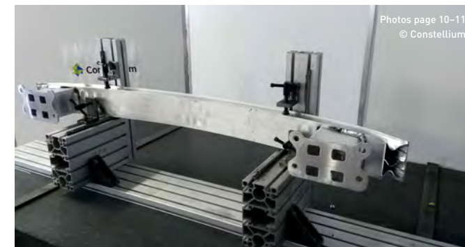
Picture 3: Crash management system prototype – Automotive Structure & Industry, Constellium R&T Center
